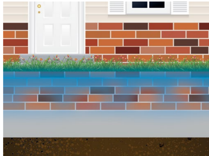
Conventional treatments have very limited movement through the soil and can be unevenly distributed within the protective zone.
